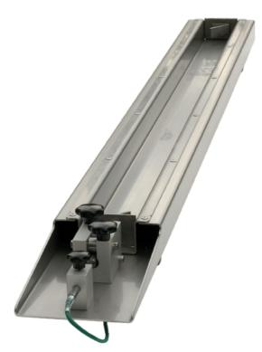
The Shrinkage Drain made of a 1m (or shorter) long ushaped stainless steel profile which contains the specimen. To avoid wall friction the drain is covered with a removable Neoprene ® sheet. On one side a removable
