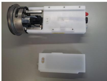
Figure 7: Mounting the battery pack: Keep the electrical contacts clean and dry.
