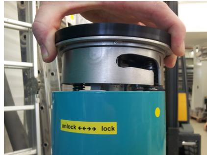
Figure 13: Turn the electronic unit until the bayonet snaps.
