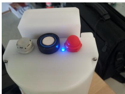
Figure 10: The power switch of the SLIPER: For Power-ON push and hold the red button on the control unit until a double beep is heard. The blue LED is blinking if a Bluetooth connection is not established. The black ring in the middle is the head of the ultrasonic distance sensor. The grey button on the far left is the vent flap.
