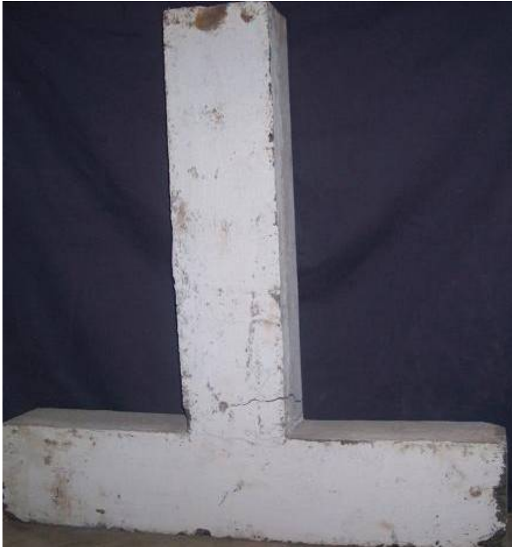
Fig. 9 Failure pattern of beam-column joint with V_f = 0.5\%
