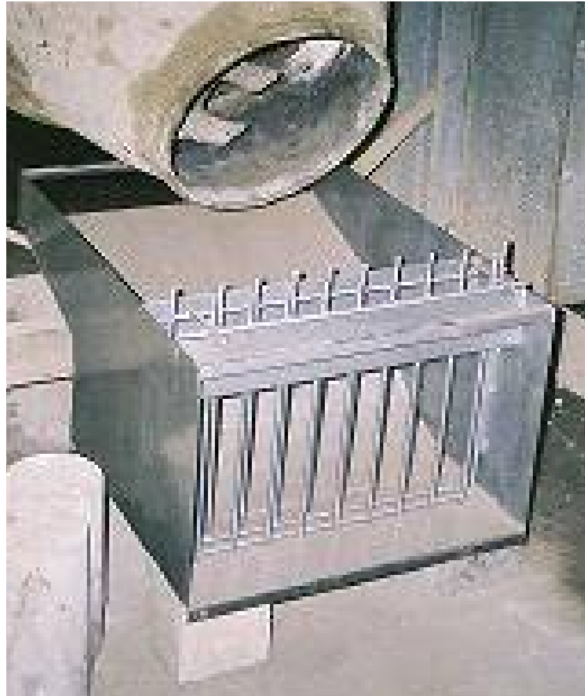
Fig. 5 Equipment for acceptance test of SCC at site
