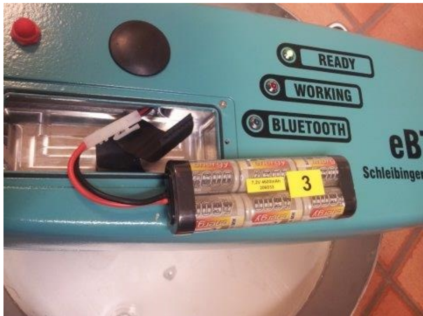
Figure 6: Put the accu pack in the right direction. Observe the space for the connector and cable.
