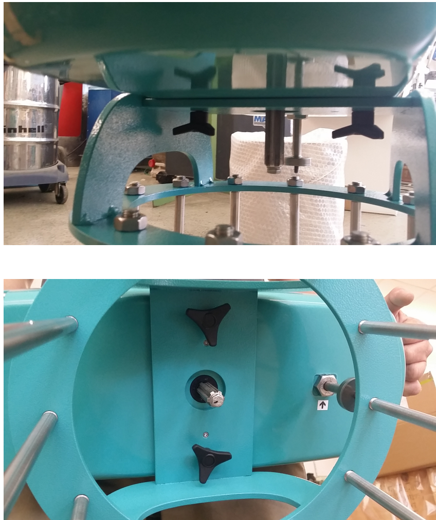
Figure 18: eBT-V - fixing of the device holder
