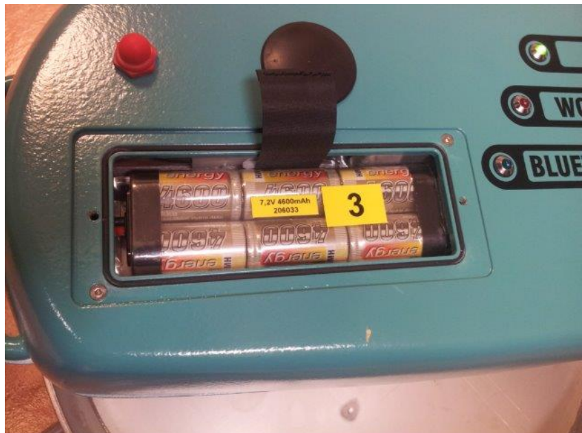
Figure 7: After placing the accu pack, make sure that the lid is waterproof mounted
