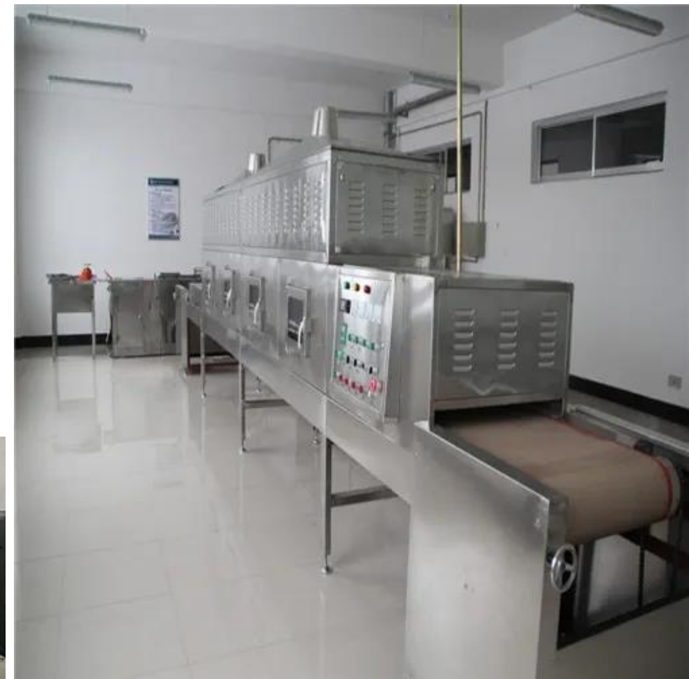
Microwave foaming equipment
