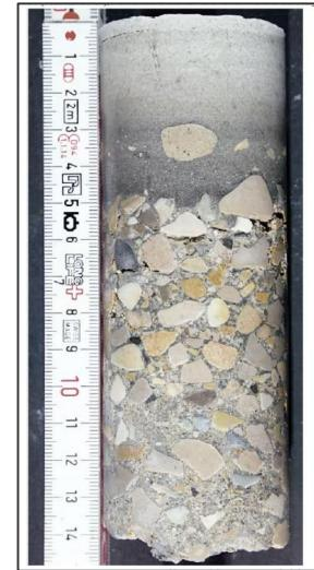
Sedimentation due to too much compaction work
