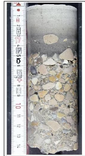
Blowholes due to insufficient compaction work
