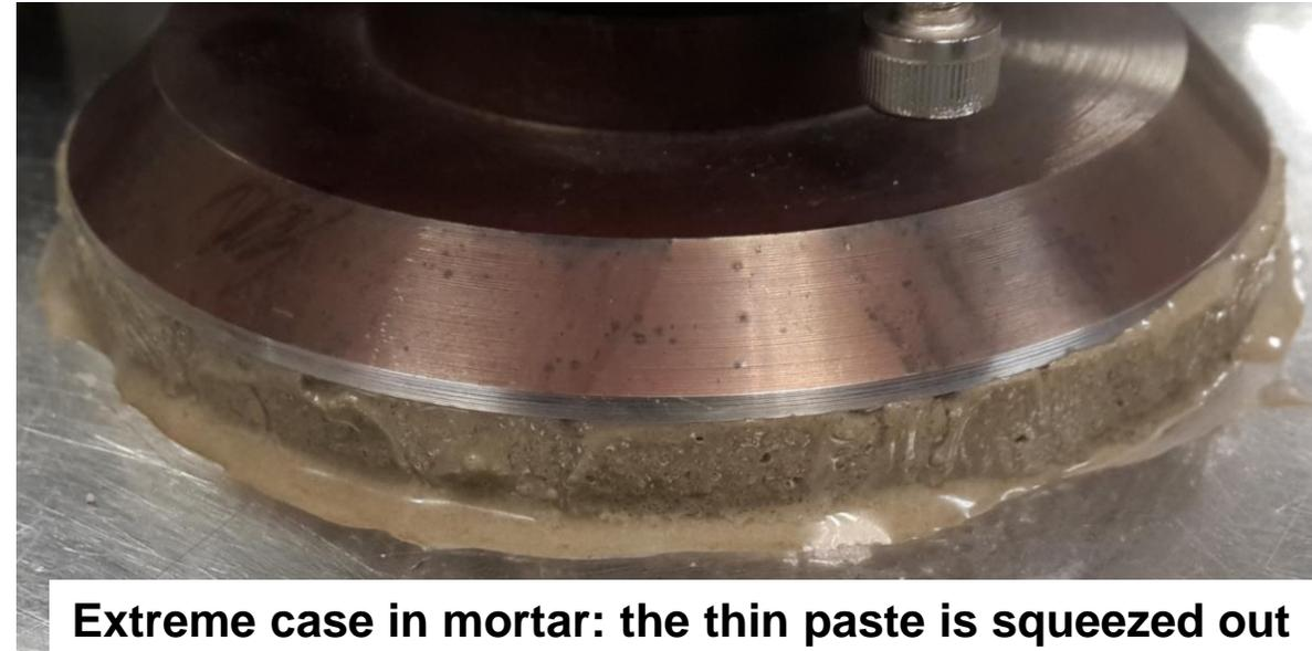
Extreme case in mortar: the thin paste is squeezed out
