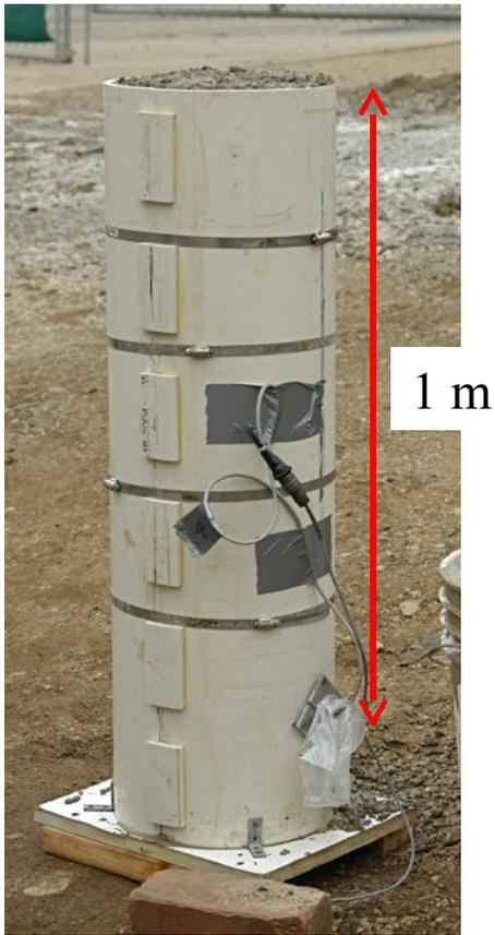
Filled quickly to generate maximum pressure
