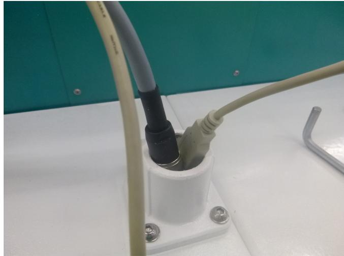
Figure 3: Thread the cables through the mounting hole
