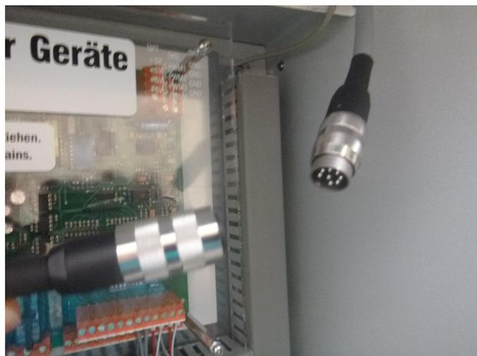
Figure 6: Connect the DIN connector and the D-Sub connector at the control unit
