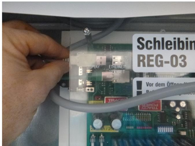
Figure 7: Connect the USB to the controll unit
