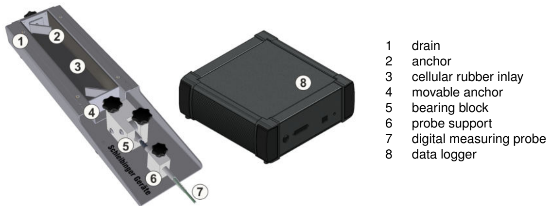
Figure 1: Components of the Shrinkage drain equipment.
