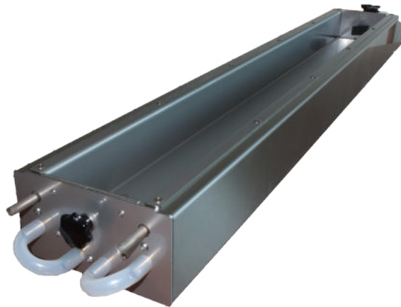
Figure 9: Shrinkage drain with the tubes for temperature control.
