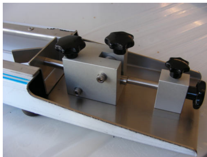
Figure 7: Fixing of the movable anchor with the fixing stamp for filling the sample.
