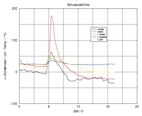
Above you see a typical data plot. The x-Axis shows the time in days, the y-axis temperature in °C and length change in microns. After 4 and half day the floor heating was activated. The green line shows the temperature at the bottom of the specimen, the blue line is the temperature in the core of the specimen. The red line shows the
