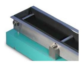
High precision measurement are guaranteed, by two static abutments and a massive u-shaped steel baseplate. A neoprene foil between the form work and the material avoids friction and blocking of material, also when expanding materials are used. The form work is static independent from the mortar beam which is supported by two well defined points.
