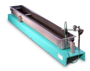
Withe the Schleibinger Bending Drain you measure the shrinkage and bending of building materials. Also you may simulate with a built in electrical heating a real world floor heating.
