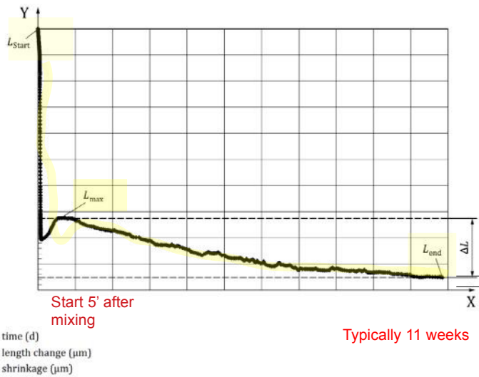
Figure A.1 — Typical length change curve of a calcium sulfate screed material
