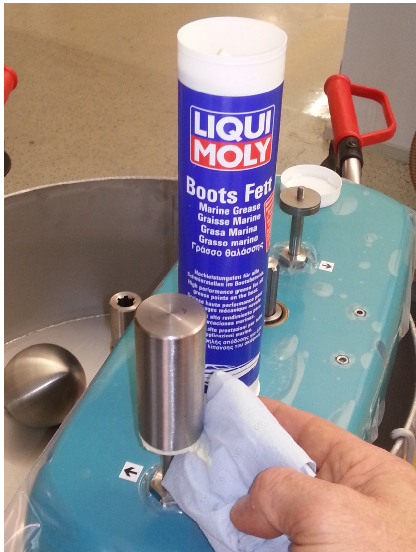
Figure 3: Screw the probe onto the sensor head. Please use no tools. Remove the remaining grease with a piece of wool or paper
