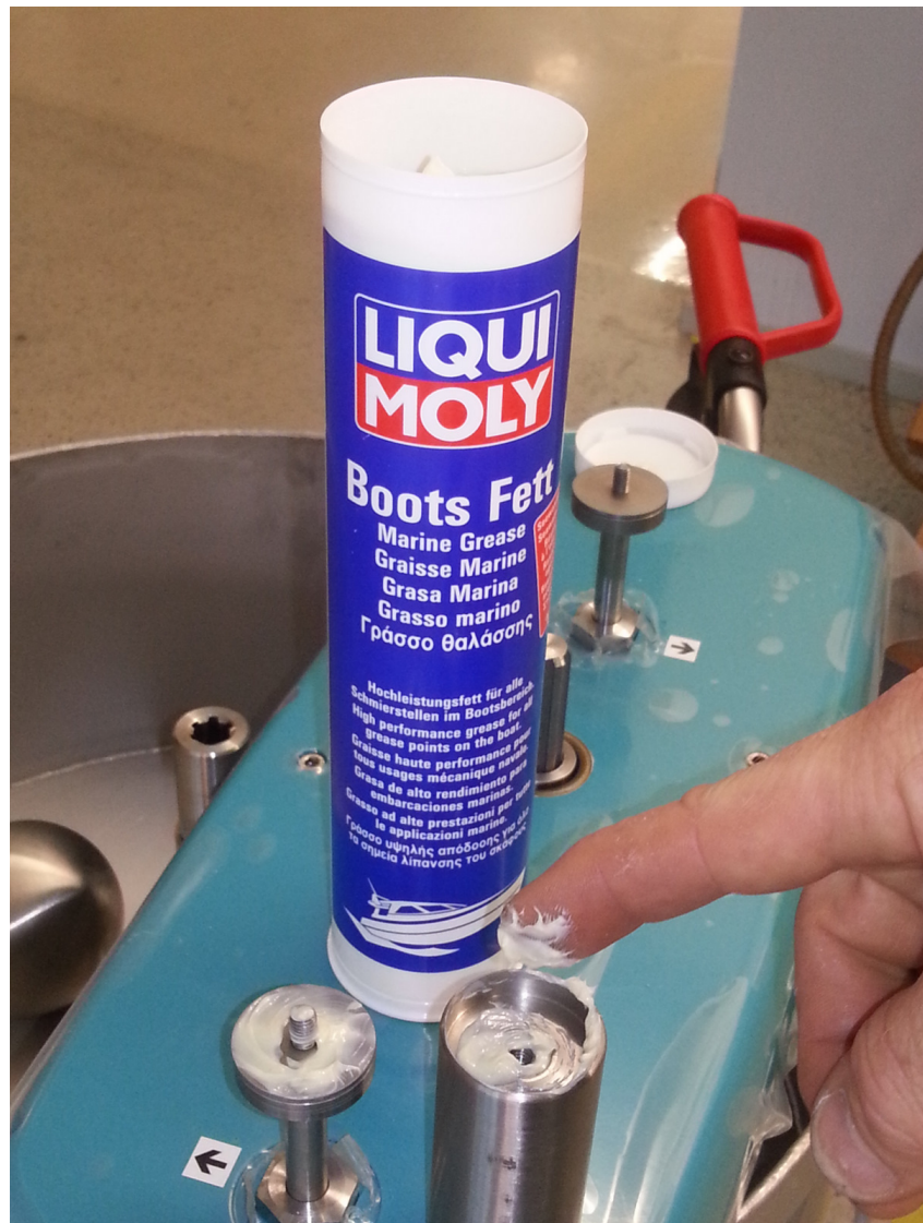
Figure 2: Seal also the thread of the probe with the the grease delivered with the eBT2
