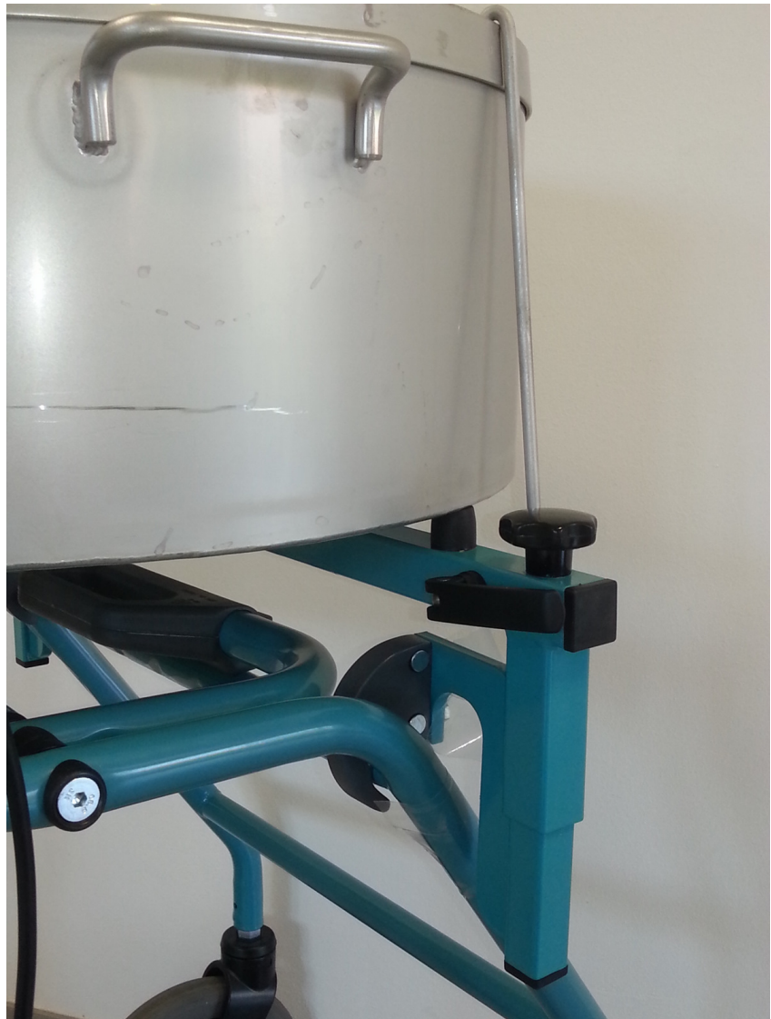
Figure 5: Fix the vessel with the two hooks.
