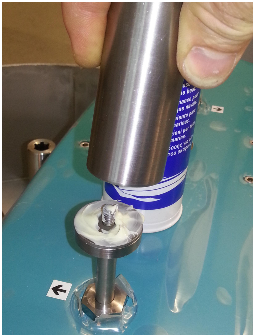
Figure 1: Seal the probe Strain Gage with the the grease delivered with the eBT2
