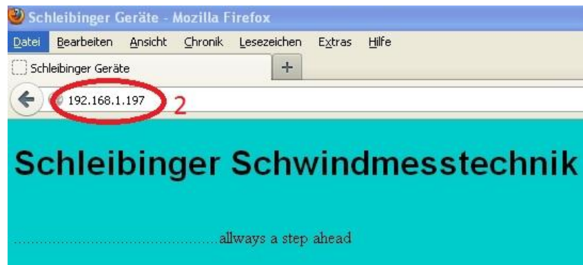
Figure 14: Accessing the data logger with a fix IP address
