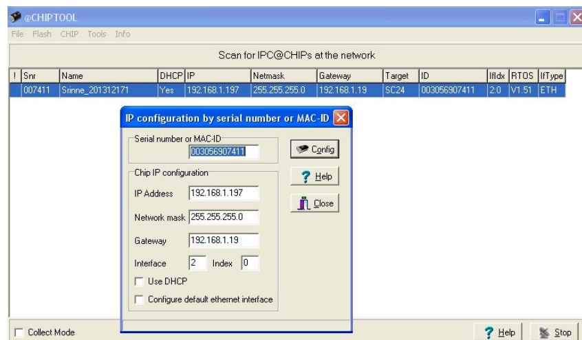
Figure 16: Configuring the data logger for a direct connection between the PC and the data logge with the program chiptool
