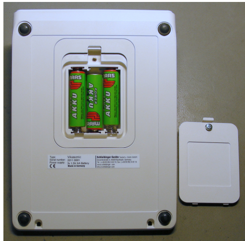
Figure 9: Opened battery compartment of the Vikasonic
