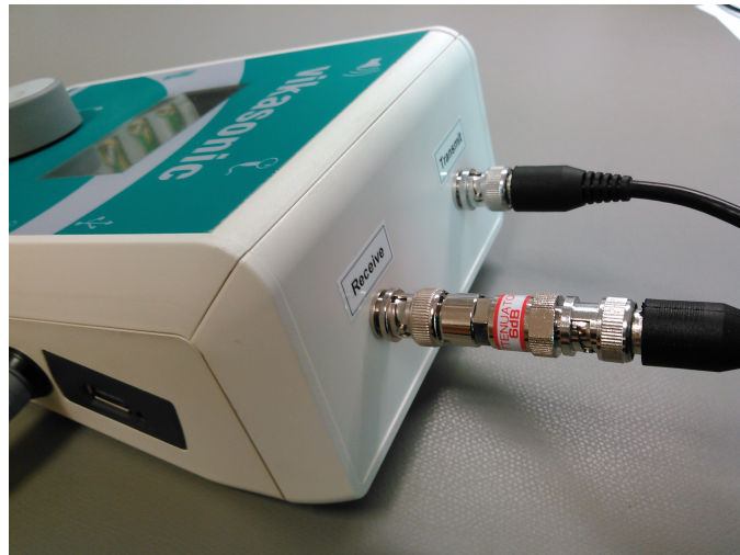
Figure 11: Connect the Measuring Bath with a 6dB attenuation element to the receiver port.
