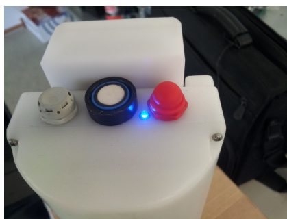
Figure 10: The power switch of the SLIPER: For Power-ON push the red button on the control unit. The blue LED is blinking if a Bluetooth connection is not established. The black ring in the middle is the head of the ultrasonic distance sensor. The grey button on the far left is the vent flap.
