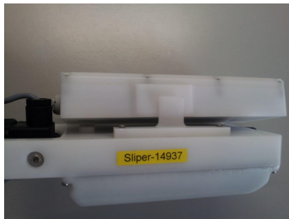
Figure 8: Insert the battery pack until the tongue snaps
