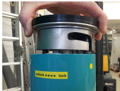
Figure 12: Turn the electronic unit until the bayonet snaps.
