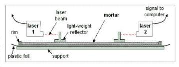
reflectors, which are placed on top of the fresh mortar. The change in distance between the reflectors is then registered with an accuracy of 0.1  $\mu$ m. The non-contact laser device allows to start measurement right after emplacement of the fresh mortar.
