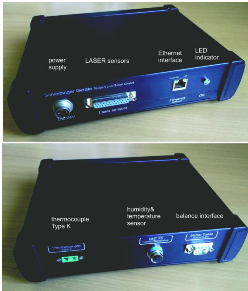
Figure 4: Data logger: front side and back side.
