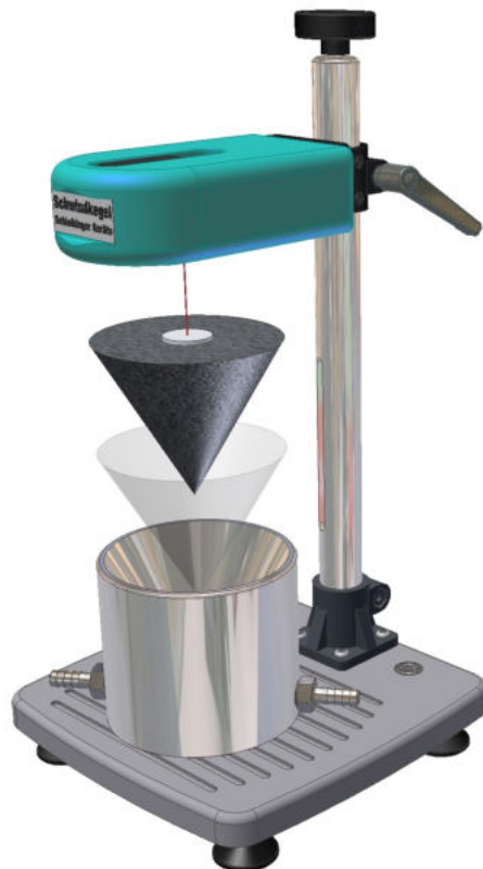
Figure 3: The Shrinkage Cone as exploded view. Cone formed sample container, partition foil, sample and reflector
