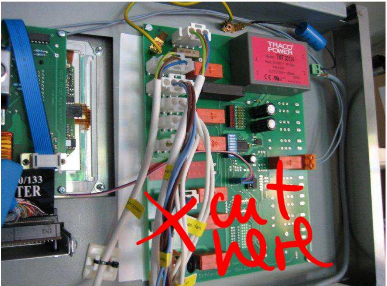
2. pull the brown wires to back to the evaporator; open all cable ties
