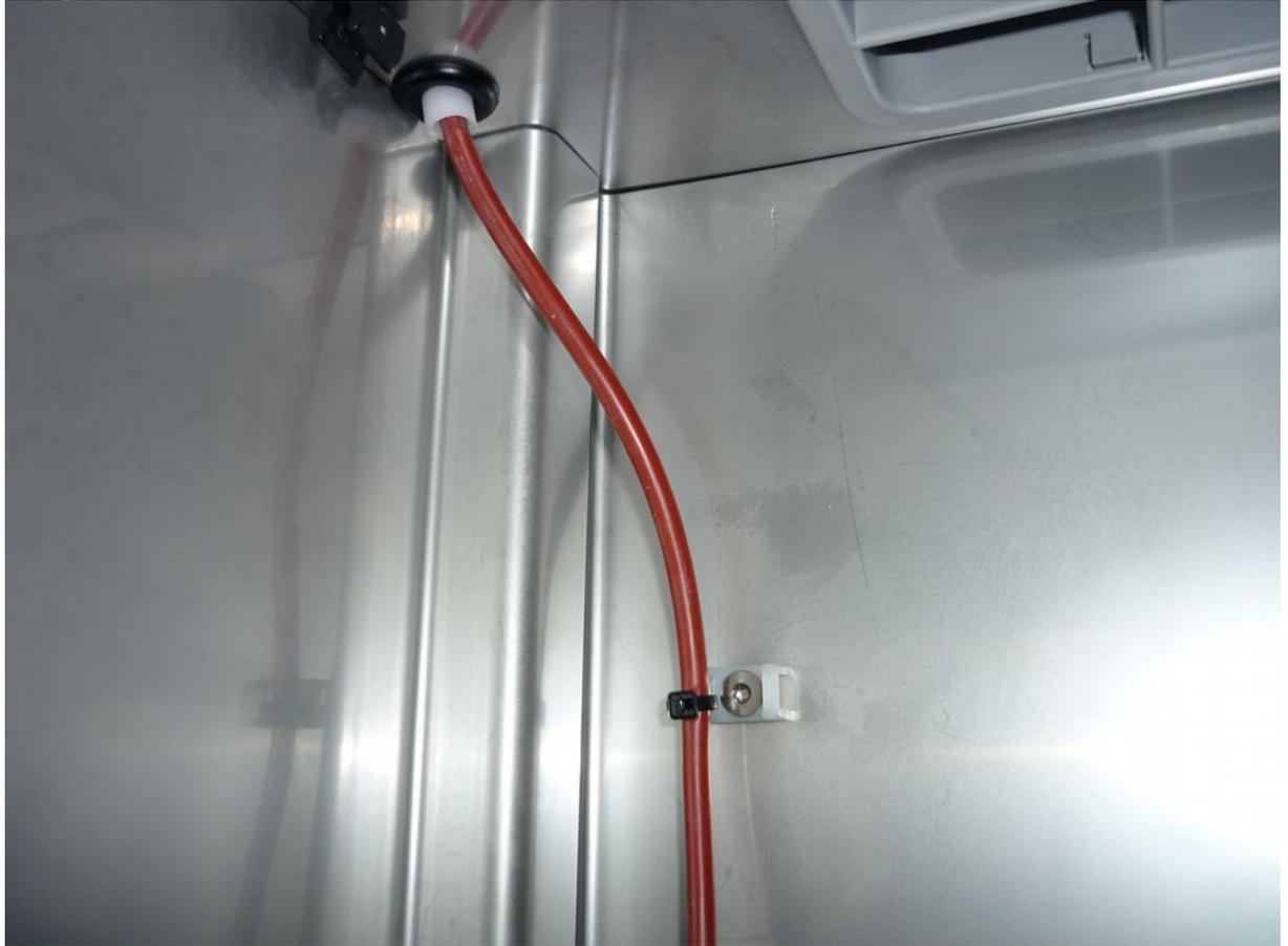
8. The cable of the spare sensor through the hole on the top of the cabinet back up and connect to the screw terminal of the controller board.
