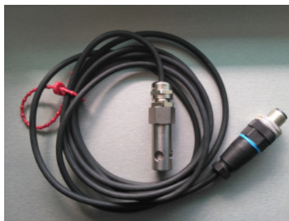
Figure 11: combined humidity and temperature sensor
