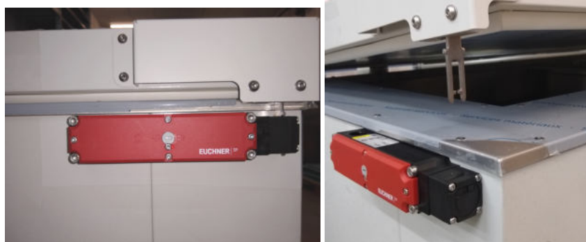
Figure 2: Lid lock on the left side of the machine: closed position (left) and open position (right).
