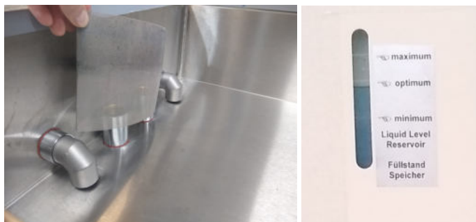
Figure 8: Inserting the filter (left) and optimum filling quantity of the heat transfer fluid of the machine (right).
