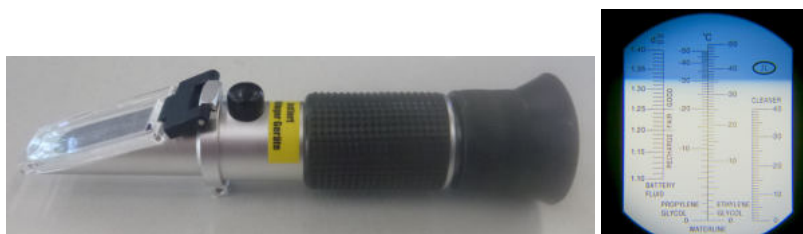
Figure 42: Refractometer (left) and antifreeze indicator at -36 °C (right).
