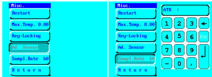
Figure 28: Sub-menu „Misc.“. with activated additional sensor (left) and input of sampling rate (right).
