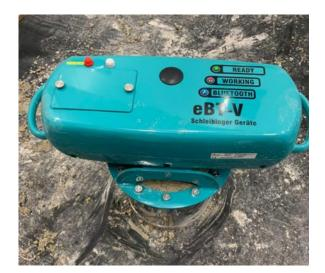
Test program conducted on a construction site in Hamburg, focusing on deep foundation testing, utilized the eBT-V rheometer and employed a step-down shear profile.
