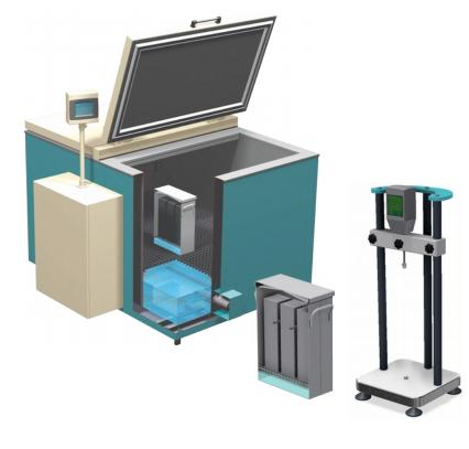
The samples will be placed into the sample container and stored in the ASR Reactor. The temperature inside the Reactor can be set very precisely in the range of room temperature to 60 °C. In addition, ASR reactor can be used as a fog chamber due to the optional fog generation system, which is recommended for the storage conditions at lower temperatures such as 38 °C or 40 °C.
