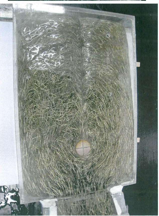
Orientation of steel fibers in hydrogel around an obstacle
