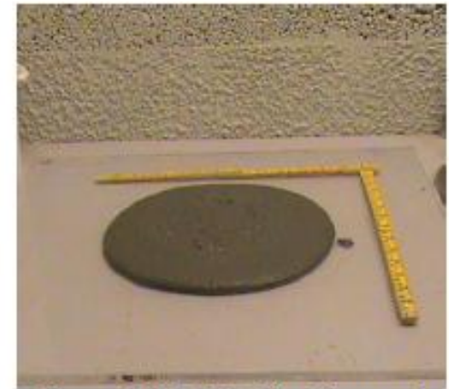
Figure 5.2.1.1.7: Mini slump of mortar produced with low yield cement
