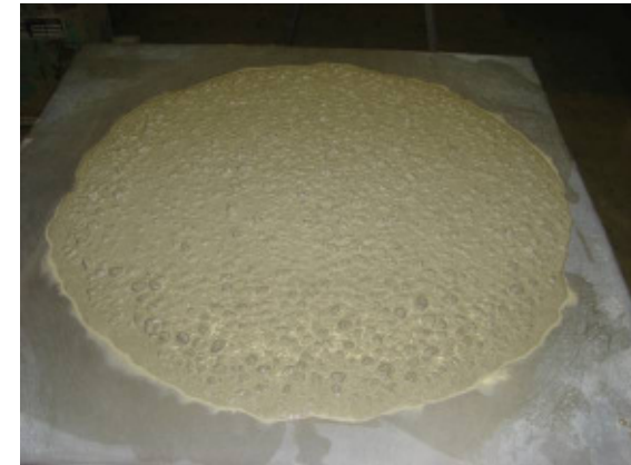
Concrete with St2 at 30 °C after 10 min.
