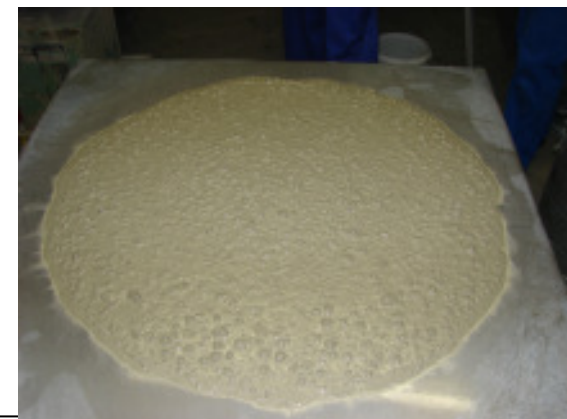
Concrete with St2 at 30 °C after 10 min.
